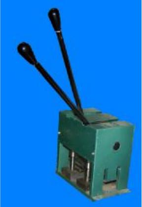
A green manual press with two black handles, used for punching holes in the bottom cornice. |
