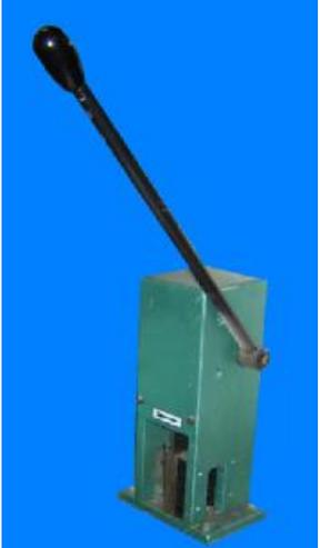
A green manual press with a black handle, used for cutting the bottom cornice.               |
